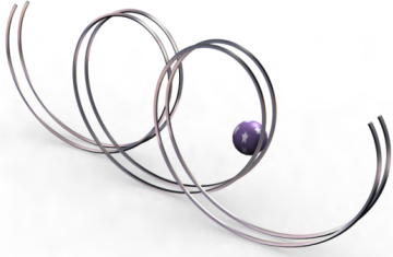
Fig. 9. Real-time simulation of a ball in a double loop. The ball initially has some spin, and different friction coefficients between the ball and the rails are tested. When friction is high, the spin energy is converted into translational kinetic energy, which makes the ball roll through the loops.
